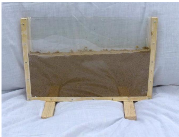
(a) A perspex-sided display cabinet for demonstrating infiltration rate in soil. The cabinet is filled with sand and water poured onto the top of the sand. The rate at which the water infiltrates into the sand and the depth to which a given depth of applied water penetrates can then be viewed.
