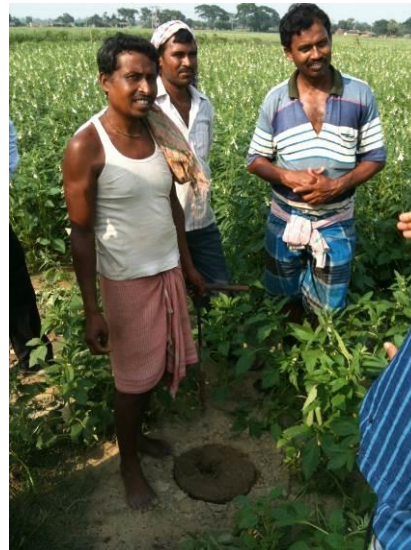
(d) All the water had infiltrated after 2 hours, surface still saturated. WUA secretary augered down through the centre to see the infiltration depth.
